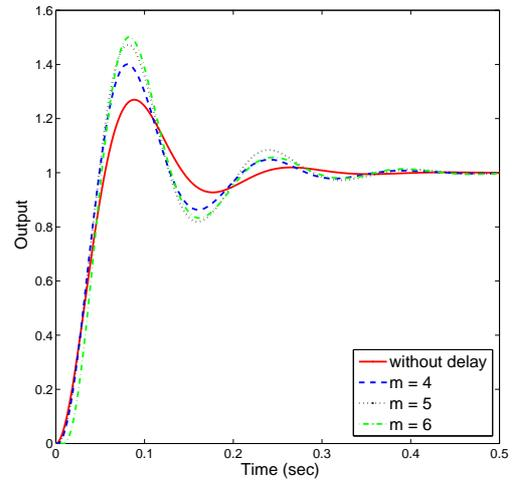
Fig. 2. Effect of the delay variance with different MAC parameters of  $m = 4, 5, 6$ .
