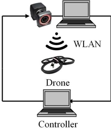
Fig. 1. CPS testbed with VICON localization system, where a drone is controlled through Wireless LAN.
