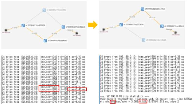
Fig. 3. Experimental results of link failover.
