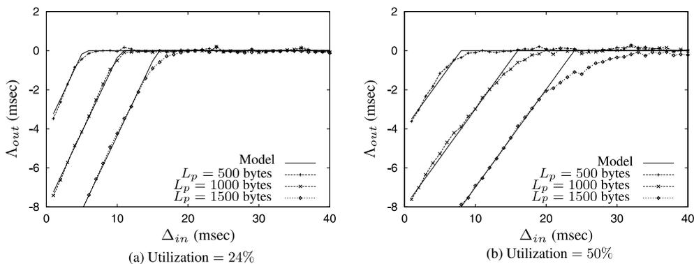
Fig. 4. Validation of the deterministic model:  $\Delta_{in} - \bar{\Delta}_{out} (= \Delta_{out})$  versus  $\Delta_{in}$ .
