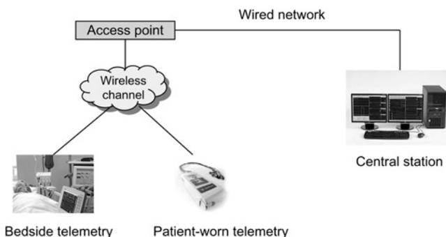
**Figure 1** Illustration of the unified medical telemetry system
