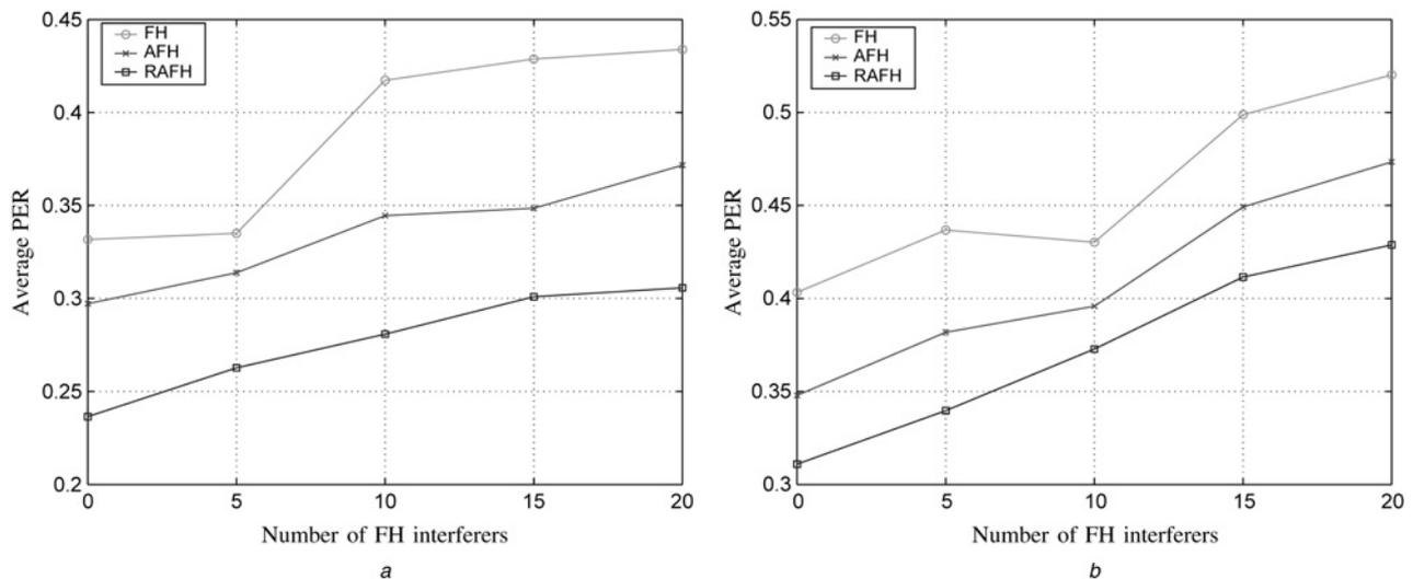
**Figure 4** Average PER vs number of FH interferers with random DS interferers
