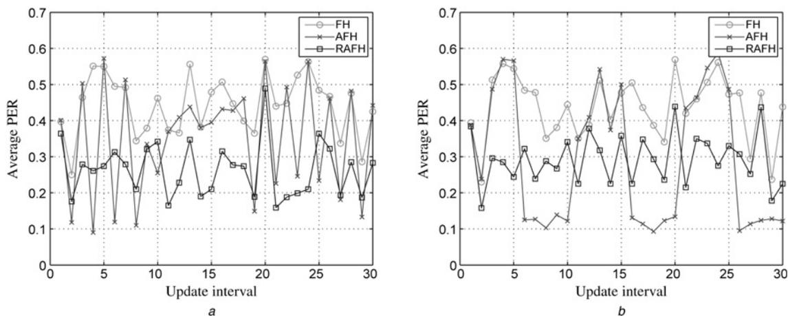
**Figure 5** Effect of the AFH reset timer  $T_s$  on PER fluctuation ( $\gamma = 0.002$ ,  $\mu = 0.001$ ,  $\eta = \xi = 0.2$  and 10 FH interferers)
