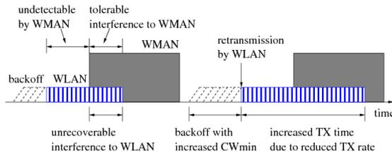
**Fig. 2** Effect of inter-system interference on channel access.
