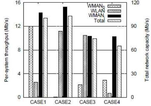
**Fig. 3.** Per-system throughput and aggregate network capacity for four cases with different carrier sensing threshold.
