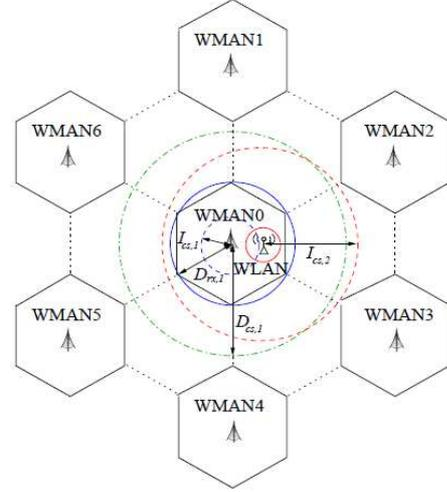
**Fig. 1.** Coexistence scenario of WMANs and WLAN.
