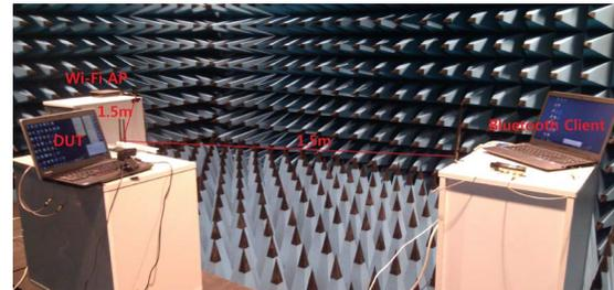
Fig. 8. Experimental environment in a RF chamber.
