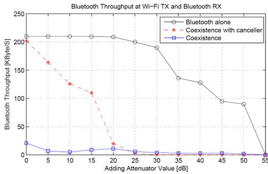
Fig. 9. Bluetooth throughput vs. channel attenuation.
