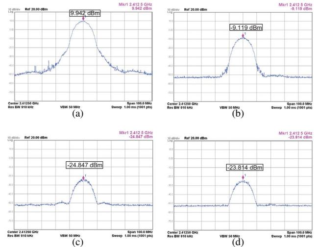
Fig. 7. Spectrum Analyzer: (a) Directly measuring the transmission signal, (b) Received interference signal after channel, (c) Received interference signal with canceller and (d) Received interference signal at 21cm distance.
