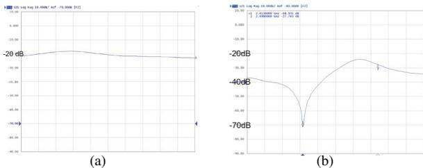
Fig. 6. Network analyzer: (a) Received interference signal and (b) received interference signal with our canceller.
