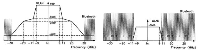
(a) AFH: Wi-Fi TX / Bluetooth RX (b) AFH: Bluetooth TX / Wi-Fi RX
