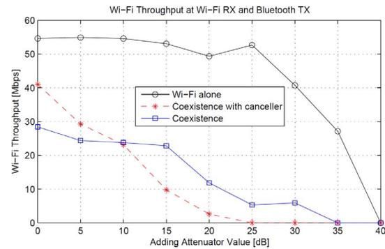
Fig. 10. Wi-Fi throughput vs. channel attenuation.
