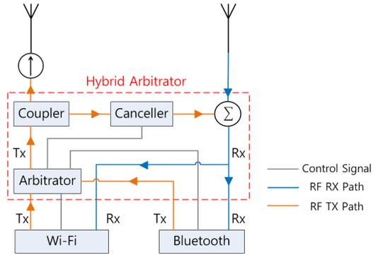
Fig. 4. A diagram of the hybrid arbitrator.
