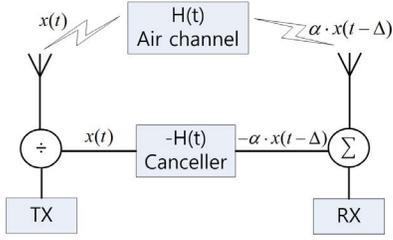
Fig. 3. A mechanism of the canceller.
