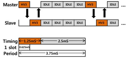
Fig. 1. SCO: HV3 packet timing.
