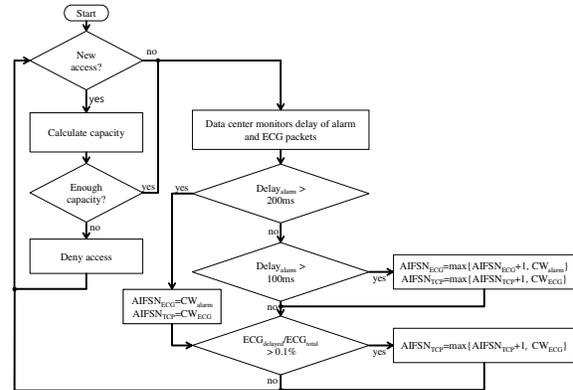
Fig. 2. Flowchart of proposed algorithm with admission control.
