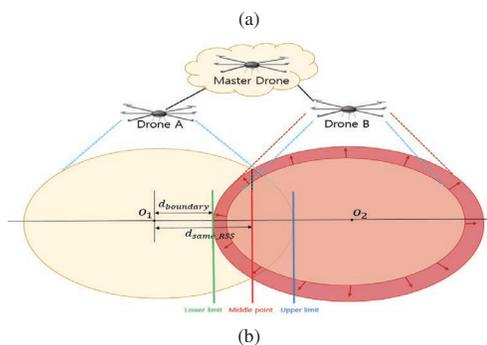
Fig. 1. Variation of the  $D_{Same\_RSS}$  as the difference of Drone's coverage increases
