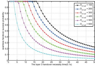
Fig. 5. Relationship between the seamless handover success probability and the L3 handover necessity time.
