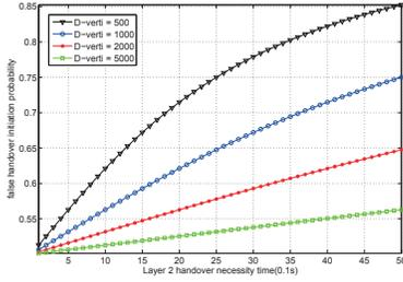
Fig. 4. Relationship between false handoff initiation probability and vertical distance of the overlapped area.
