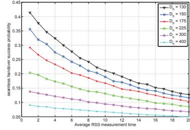
Fig. 6. Relationship between average RSS measurement time and the seamless handover success probability.
