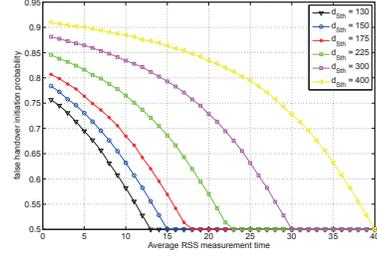
Fig. 7. Relationship between average RSS measurement time and false handover initiation probability.
