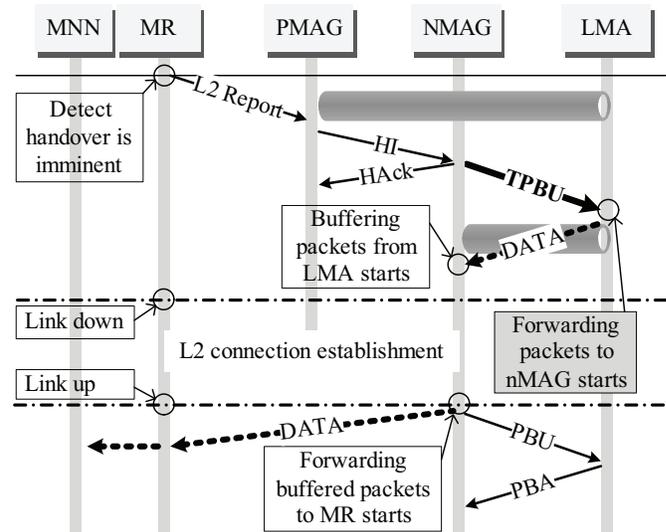
Fig. 3. The handover operation of IFP-NEMO.
