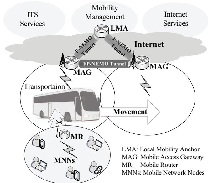
Fig. 1. Architecture overview of PMIPv6-based NEMO.
