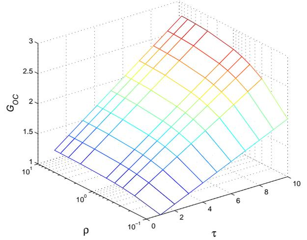
Fig. 5. The relative overall cost gain ( $N_{MNN} = 10$  and  $\omega = 0.2$ ):  $G_{OC}$  vs. the weight factor of tunneling,  $\tau$ , and the session to mobility ratio,  $\rho$ .
