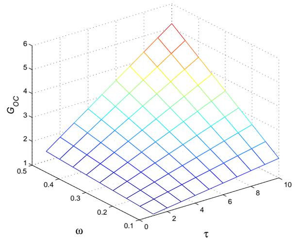
Fig. 6. The relative overall cost gain ( $N_{MNN} = 10$  and  $\rho = 1$ ):  $G_{OC}$  vs. the weight factor of tunneling,  $\tau$  and the ratio of using indirect path,  $\omega$ .
