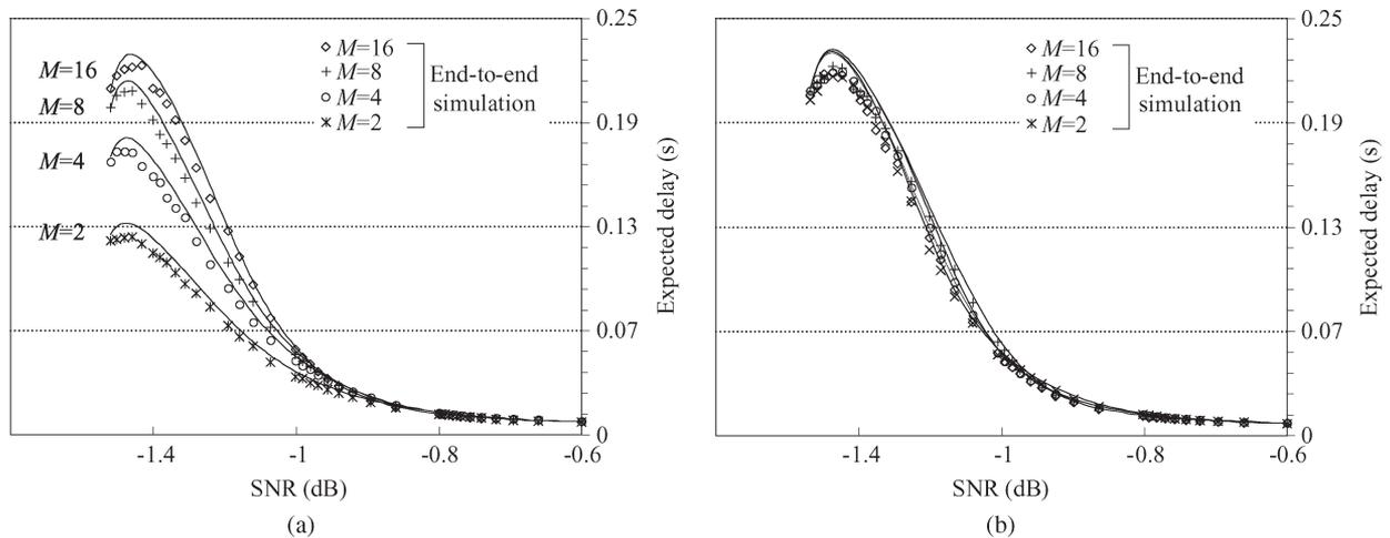
Fig. 5. Expected delay incurred in RS decoding of a single ECB subblock. (a) 2 m/s ( $f_D' = 0.01$ ). (b) 20 m/s ( $f_D' = 0.1$ ).
