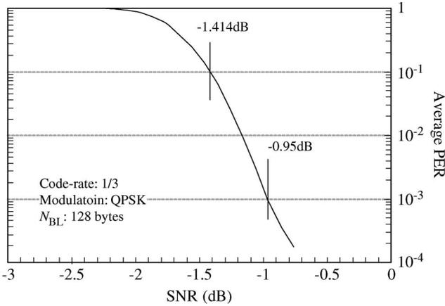
Fig. 4. Effect of turbo coding on the average PER for varying values of the SNR.
