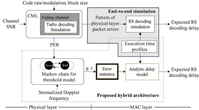
Fig. 3. Hybrid framework for analyzing the MAC-layer delay in mobile receivers.
