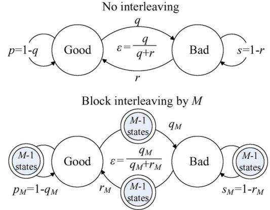
Fig. 1. Representation of the error process by a state diagram with Markov parameters.
