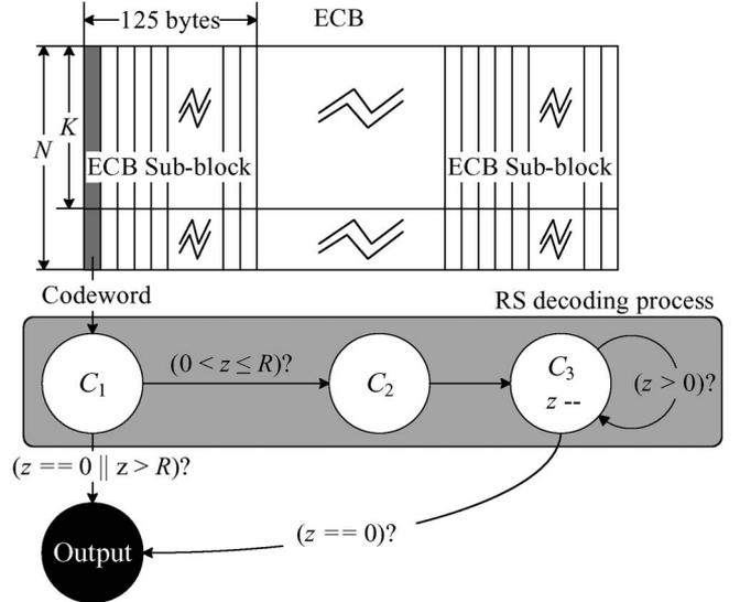
Fig. 2. Computational components  $C_1$ ,  $C_2$ , and  $C_3$  of the RS decoding process.
