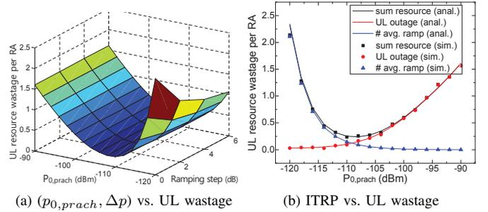
Fig. 4: Effect of PRACH power on uplink wastage.
