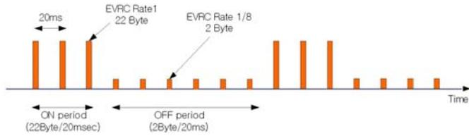
Figure 11: VoIP EVRC Payload Model
