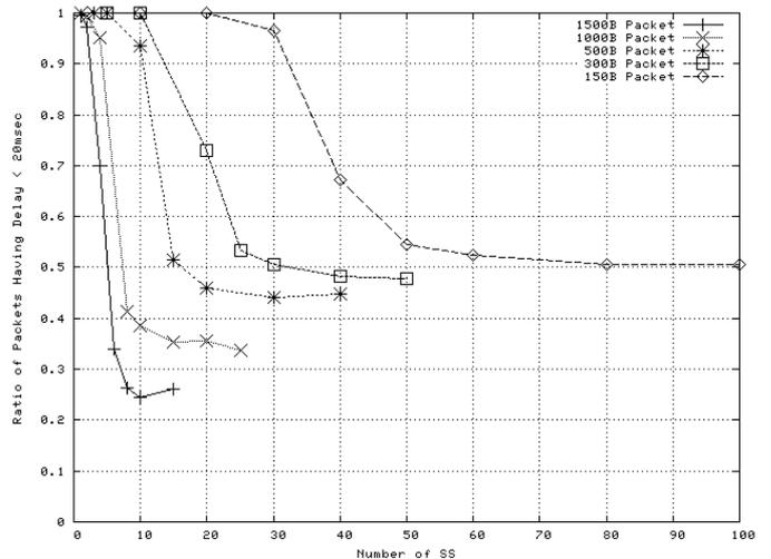
Figure 10: Ratio of Packets Having Less Than 20ms Delay
