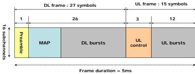
**Figure 1: WiBro OFDMA TDD Frame Structure**
