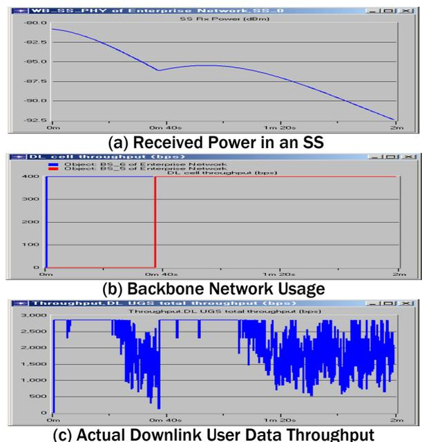
Figure 7: Example Downlink Hand-Over Trace
