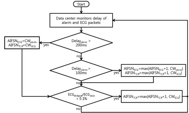
Fig. 2. Proposed algorithm for tuning the AIFS value.
