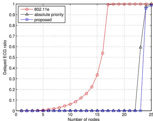
Fig. 4. Ratio of delayed ECG packets over total received ECG packets.
