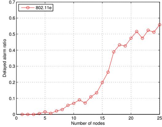
Fig. 1. Ratio of delayed alarm packets over total received alarm packets.
