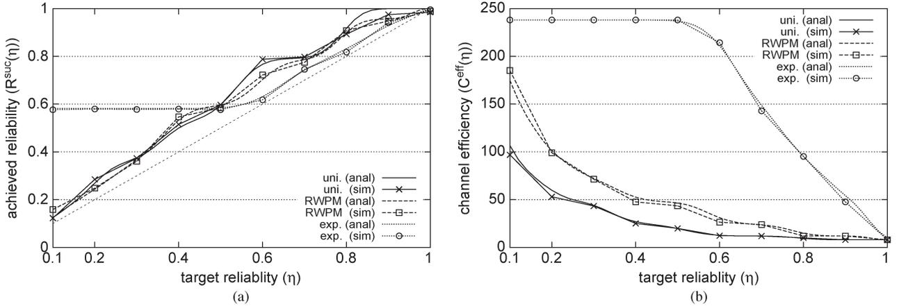
Fig. 4. Effect of target reliability ( $\eta$ ) on the (a) achieved reliability ( $\bar{R}^{\text{suc}}$ ) and (b) channel efficiency ( $\bar{C}^{\text{eff}}$ ).
