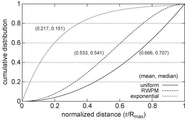
Fig. 3. Cumulative distribution and statistics of the normalized distance between the BS and the MS.
