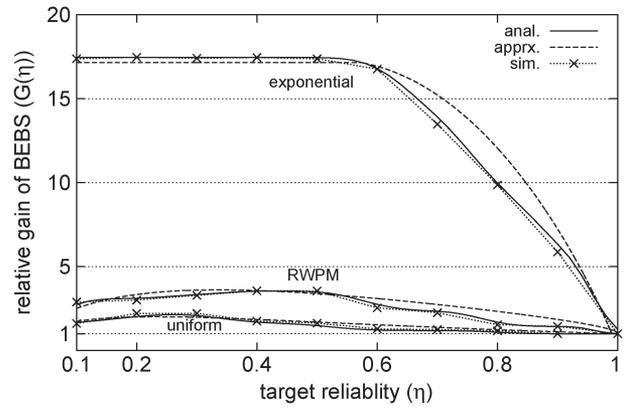
Fig. 5. Relative capacity gain of BEBS, compared with full reliable broadcasting.
