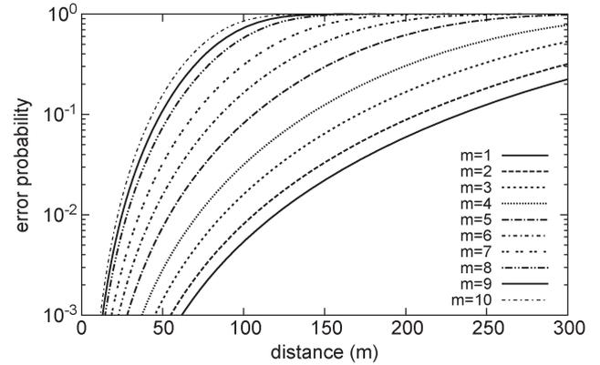
Fig. 2. Average error probability of  $B$ -bits burst ( $\bar{p}_m^e$ ) versus distance between the BS and the MS ( $r$ ).
