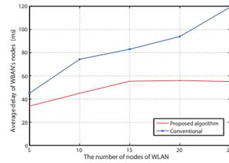
Fig. 3. Average packet delay of WBAN with respect to the number of WLAN nodes when there are 20 WBAN nodes.
