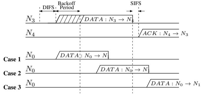
Fig. 2. Timing diagrams for two concurrent transmissions under IEEE 802.11 DCF with an RTS/CTS exchange. The transmission from  $N_3$  interferes with the data reception at  $N_1$  in Cases 1 and 2.
