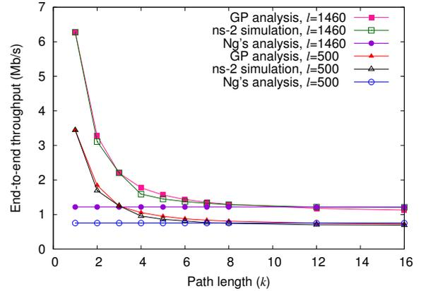
Fig. 5. Comparison of maximum end-to-end throughput for the analysis, ns-2 simulation, and Ng's analysis in [14] ( $\beta = 4$ ).
