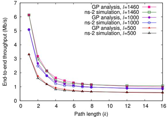
Fig. 4. Maximum end-to-end throughput for payload sizes of 500, 1000, and 1460 bytes ( $\beta = 3.3$ ).
