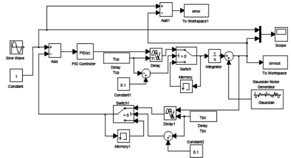
Fig. 7. Typical Simulink Model of Networked Control
