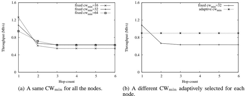
Figure 2: Throughput performance of a 6-hop wireless path for a fixed, single  $CW_{min}$  and an adaptively selected  $CW_{min}$ . (The throughput at the last hop-count is the end-to-end throughput of the multihop wireless path.)
