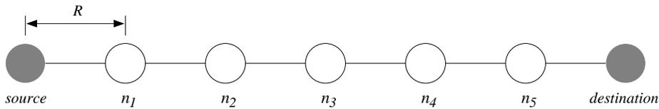
Figure 1: A multihop wireless path consisting of a source node, a destination node, and five relay nodes.
