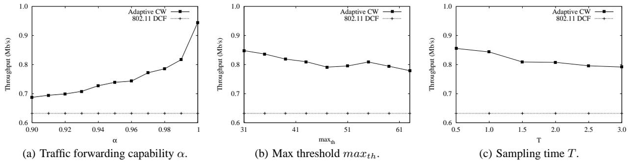
Figure 4: Throughput results with respect to the parameters ( $\alpha$ ,  $max_{th}$ , and  $T$ ) in the chain topology.
