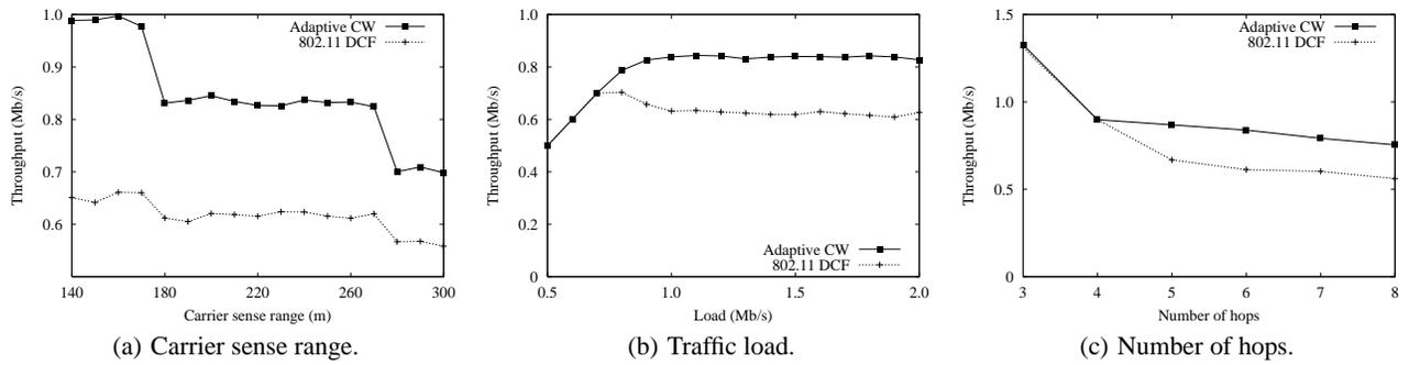
Figure 5: End-to-end throughput results with respect to the carrier sense range, the offered load, and the number of hops in the chain topology.
