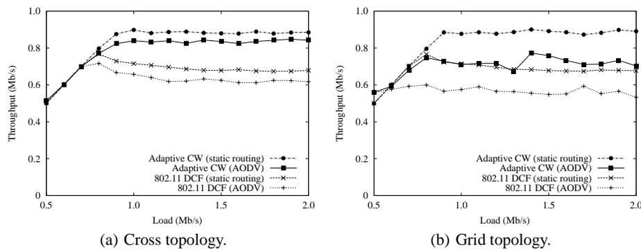
Figure 6: The aggregate throughput results with respect to the offered load in the cross and grid topologies.
