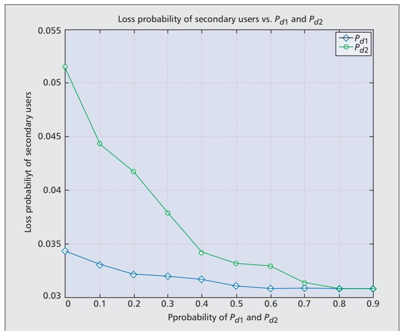
Figure 6. Effects of  $P_{d1}$  and  $P_{d2}$  on the loss probability of secondary users.
