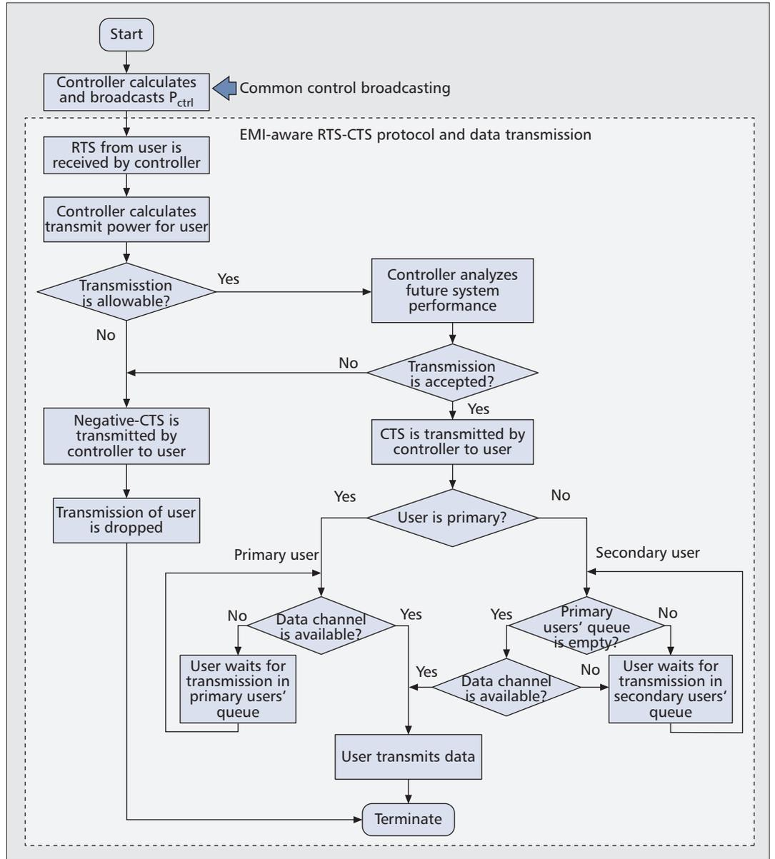
Figure 2. Flowchart of the channel access mechanism.
