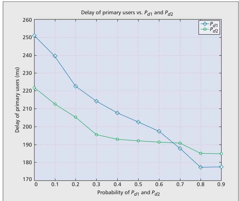
Figure 5. Effects of  $P_{d1}$  and  $P_{d2}$  on the average transmission delay of primary users.
