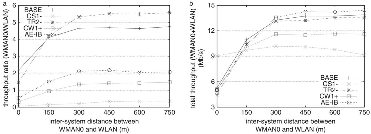
**FIGURE 10.** Performance comparison of several approaches with different degree of overlapping deployment between WMAN0 and the WLAN. (a) Throughput ratio ( $\gamma_{ratio}$ ) and (b) total throughput ( $\eta_{eff}$ ).
