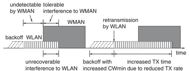
**FIGURE 2.** Responses of WMAN and WLAN to inter-system interference.
