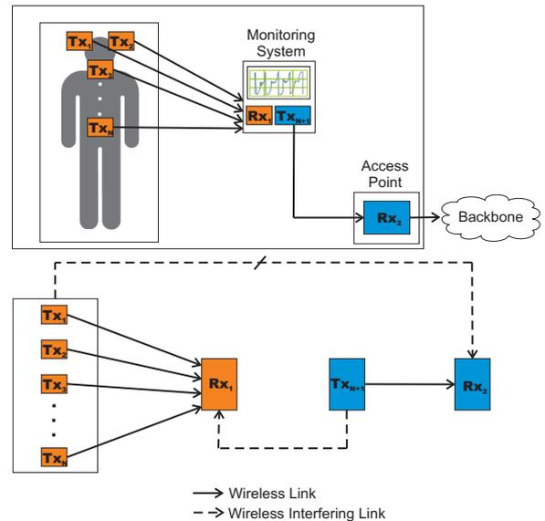
Fig. 1. Example of network topology in monitoring application at hospital room (above), and schematic of generic coexistence environment considered (below).
