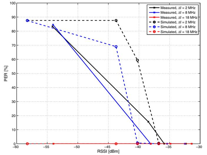
Fig. 5. Node TOPOLOGY A. PER as function of RSSI for different 802.11g carrier frequency offsets.
