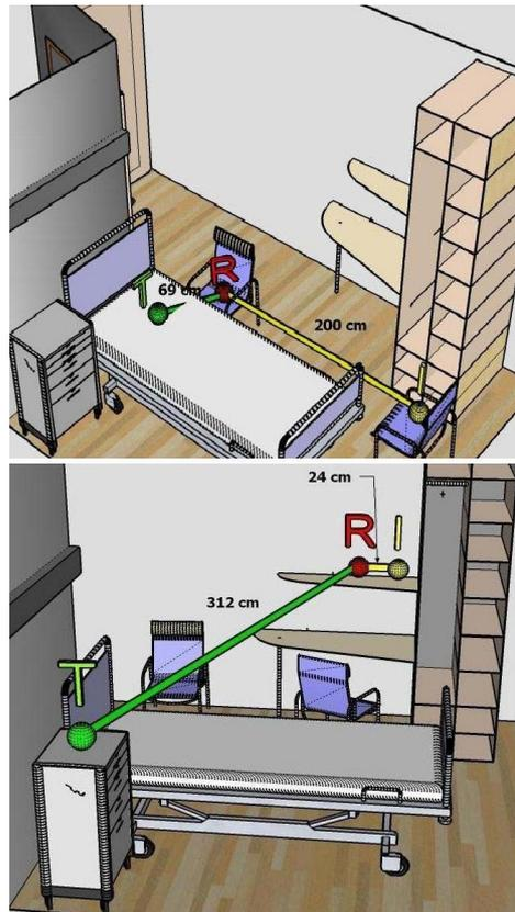
Fig. 4. Node Topology A (above) and node Topology B (below). LOS channel between transmitter and receiver, and also between interferer and receiver.
