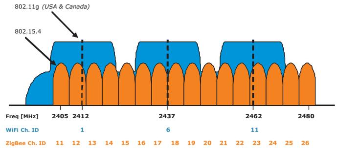
Fig. 2. Frequency channel plan for IEEE 802.11g and IEEE 802.15.4.
