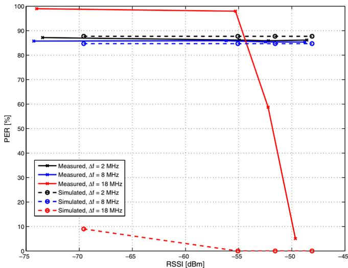
Fig. 6. Node TOPOLOGY B. PER as function of RSSI for different 802.11g carrier frequency offsets.
