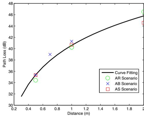
Fig. 3. Path losses for different LOS scenarios and the obtained curve fitting.
