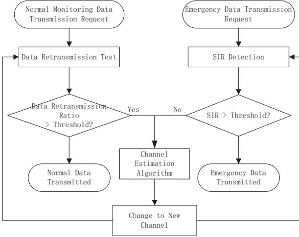
Fig. 6. Flowchart of the proposed Interference Avoidance Strategy for WeHealth
