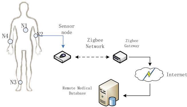
Fig. 1. Architecture of the WeHealth monitoring system
