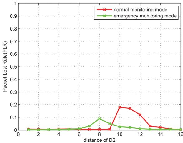
Fig. 7. PLR of the transmission in normal and emergency mode with interference avoidance strategy
