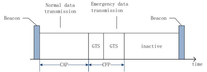
Fig. 2. Superframe of the WeHealth monitoring system
