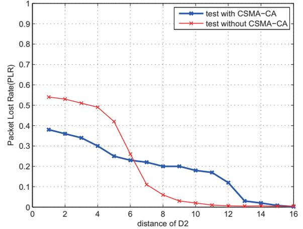
Fig. 5. PLR with different value of D2, WiFi at channel 5, and Zigbee at channel 16
