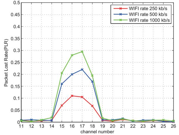
Fig. 4. PLR of Zigbee channels under WiFi channel 5 at the WiFi interference rate of 250, 500 and 1000 kb/s
