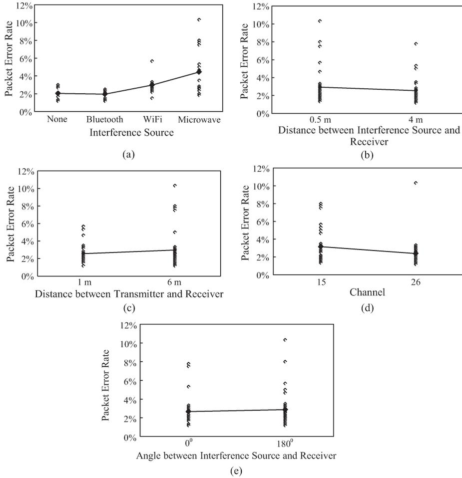
Fig. 7. PER results for experiments. (a) PER versus different ISs. (b) PER versus distances between IS and Rx. (c) PER versus distances between Tx and Rx. (d) PER versus IEEE 802.15.4 channels. (e) PER versus  $\theta$ .
