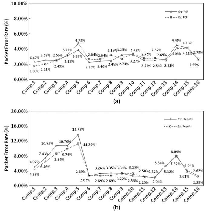
Fig. 12. Comparison results of experimental results and estimated results under Wi-Fi interference. (a) PER comparison result under Wi-Fi Interference. (b) PER comparison result under microwave oven interference.
