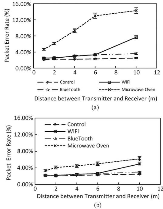
Fig. 9. PER as a function of distance between Tx and Rx. (a)  $D_{IS-Rx} = 0.5$  m. (b)  $D_{IS-Rx} = 4$  m.
