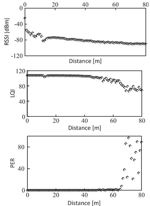
Fig. 5. Wireless signal metrics as functions of distance for Tx-Rx pair on grass.
