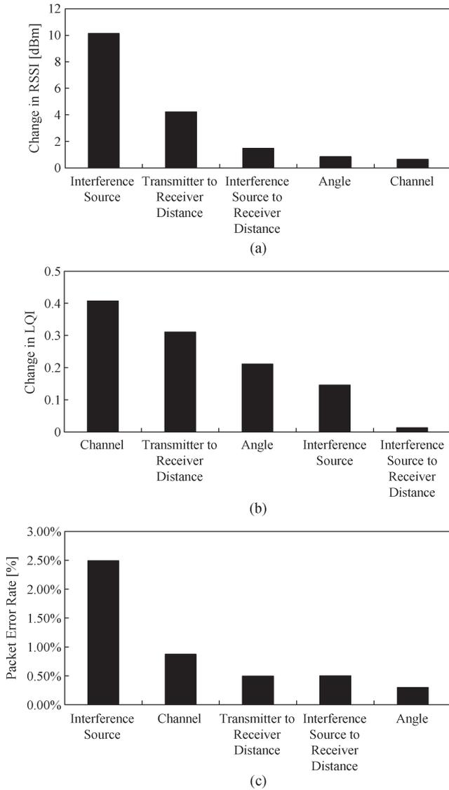
Fig. 8. Difference in RSSI, LQI, and PER between the highest and lowest levels for each factor. (a) Difference in average RSSI between the highest and lowest levels for each factor. (b) Difference in average LQI between the highest and lowest levels for each factor. (c) Difference in average PER between the highest and lowest levels for each factor.
