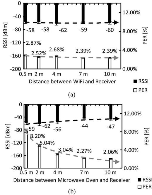
Fig. 11. PER as a function of distance between IS and Rx and IEEE 802.15.4 channel. (a) Wi-Fi as IS. (b) Microwave as IS.
