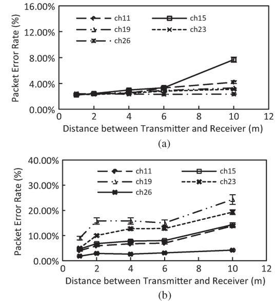
Fig. 10. PER as a function of distance between Tx and Rx and IEEE 802.15.4 channel. (a) PER distribution under Wi-Fi interference impact with  $D_{IS-Rx} = 0.5$  m. (b) PER distribution under microwave oven interference with  $D_{IS-Rx} = 0.5$  m.
