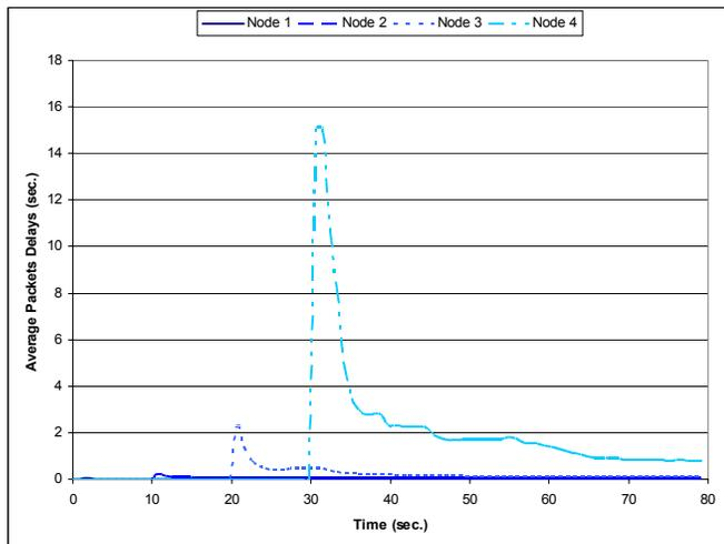
Fig. 9. Packet Average Packets End to End delay in Adaptive EDCA.
