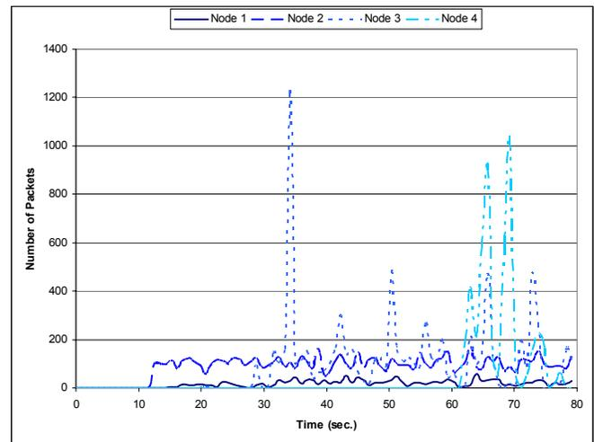
Fig. 8. Packet Drop Rate in Adaptive EDCA.
