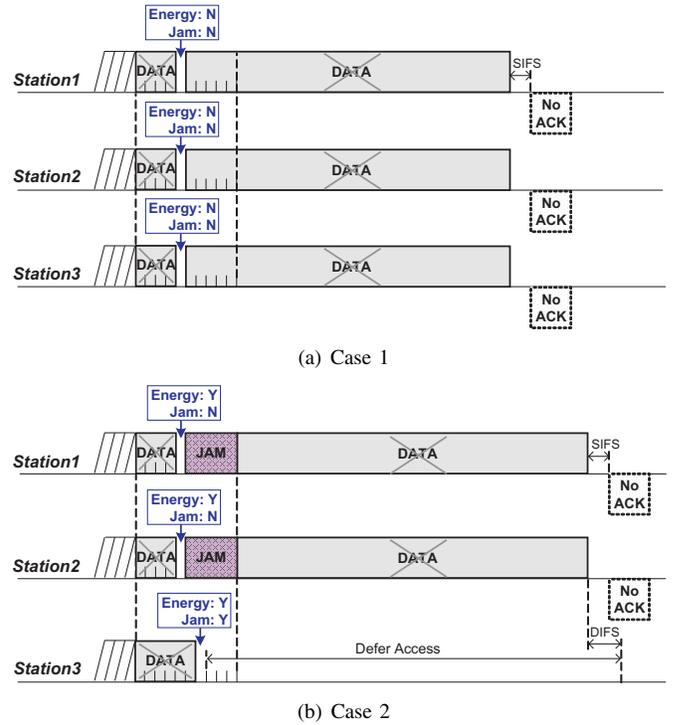
Fig. 4. Operations of CSMA/CR in two cases that a collision is not detected.
