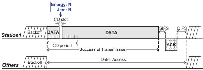
Fig. 2. Operation of CSMA/CR when no collision occurs.
