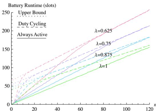
Fig. 13. When  $b_{buf} = t_{sat} = 1$ , we plot of the upper bound  $\frac{n+m-1}{1-e^{-\lambda}}$ , along with the battery runtime of always-active case  $W_{40}^0(n)$ , and the duty cycling case  $B_{40}^0(n)$ .
