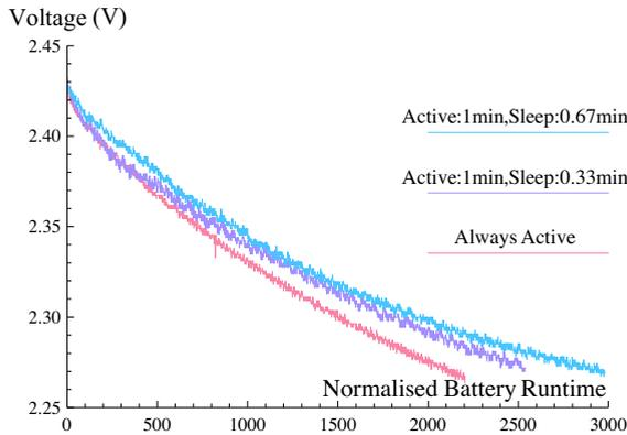
Fig. 5. The discharge profiles of Imote2 in deterministic duty cycle schedules of radio transceiver w.r.t. different sleep time periods.
