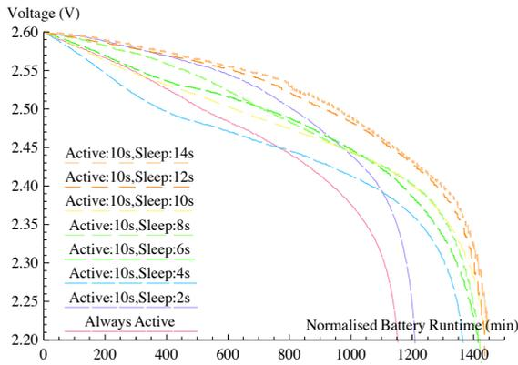
Fig. 1. The discharge profiles of TelosB in deterministic duty cycle schedules of radio transceiver w.r.t. different sleep time periods.
