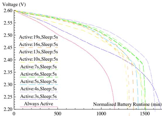
Fig. 3. The discharge profiles of TelosB in deterministic duty cycle schedules of radio transceiver w.r.t. different active time periods.
