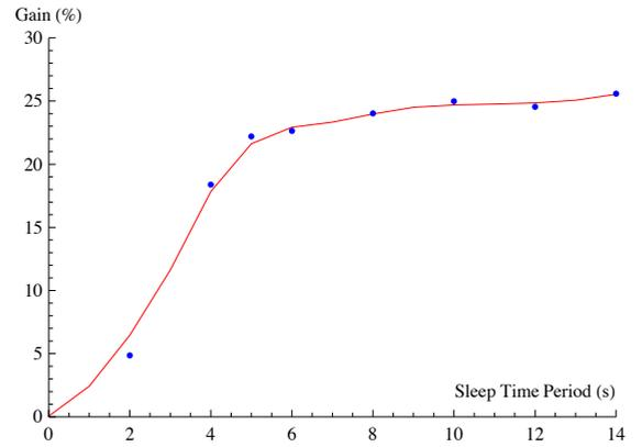
Fig. 2. The gain of normalised battery runtime of Fig. 1, as compared to the continuous (always active) radio operation.
