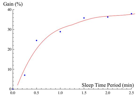
Fig. 6. The gain of normalised battery runtime of Fig. 5, as compared to the continuous (always active) radio operation.
