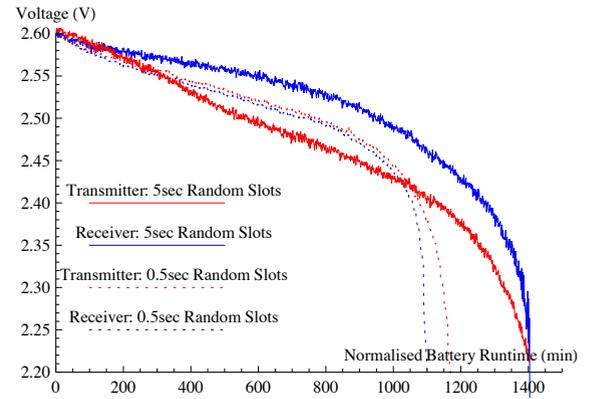
Fig. 8. Two discharge profiles a pair of transmitter-receiver of TelosB in pseudo-random duty cycle schedules of radio transceiver (duty cycle rate as 0.5): one sets each random slot as 0.5 sec, while another sets each random slot as 5 sec.
