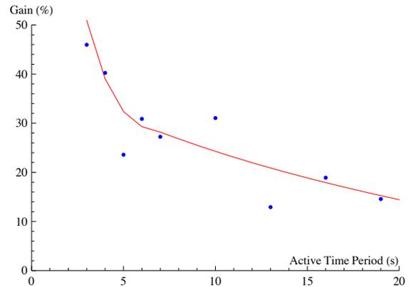
Fig. 4. The gain of normalised battery runtime of Fig. 3, as compared to the continuous (always active) radio operation.
