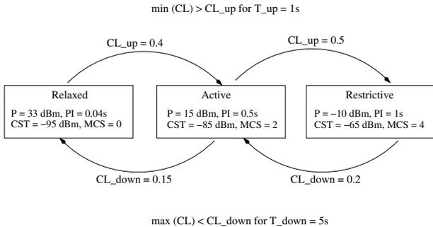
**Figure 5: The state machine proposed by ETSI DCC framework. It consists of three states and associated transmit parameters and state transition rules. When the CL is too high, the DCC algorithm tends to change all three parameters simultaneously to ease the congestion.**
