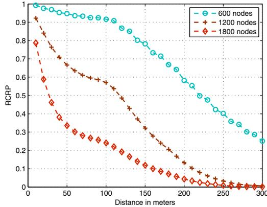
Figure 2: Packet reception performance of plain IEEE 802.11p - the x-axis is tx-rx distance and the y-axis is the ratio of correctly received packets (RCRP).
