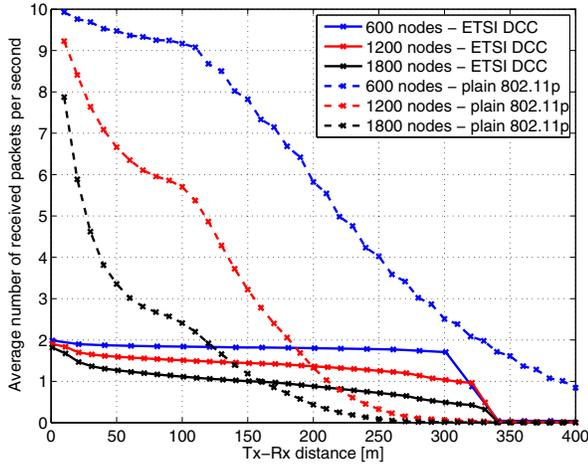
**Figure 7: Average absolute number of received packets per second as a function of the transmitter-receiver distance**
