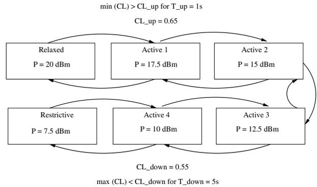
**Figure 8: State machine with six states for adapted TPC scheme**
