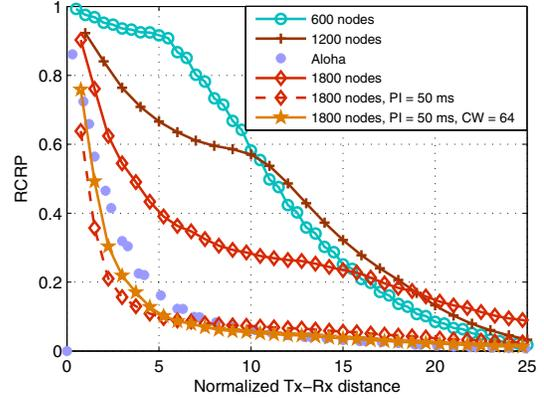
Figure 3: Discoverability performance of 802.11p: the x-axis is distance/inter-car-spacing (normalized distance) and the y-axis is the ratio of correctly received packets (RCRP). PI = 50 ms is a scenario where only 50 ms out of every 100 ms is allowed for broadcast.
