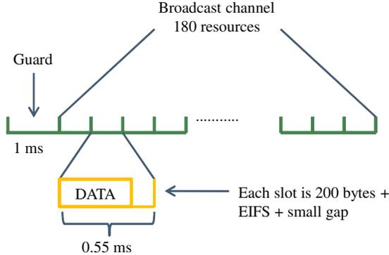
**Figure 10: Time domain structure of the channel**
