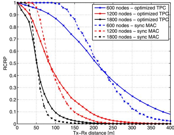
Figure 13: Comparison between the optimized TPC scheme and the sync MAC. The sync MAC performs better than the optimized TPC especially at close ranges.
