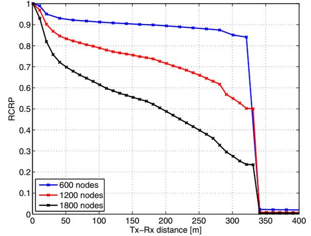
**Figure 6: Packet reception rate versus distance for ETSI DCC**
