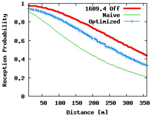
Figure 16 Safety message reception vs. distance, 150Byte, 400m, 3Hz
