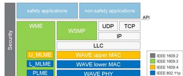
Figure 3, DSRC standards and communication stack
