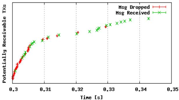
Figure 13 Safety message collisions and receptions over a CCH interval
