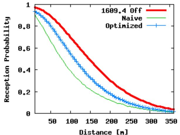
Figure 12 Safety message reception vs. distance, 75Byte, 200m, 10Hz
