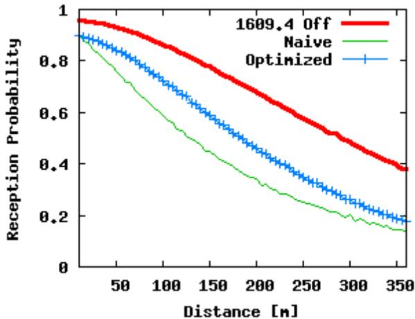
Figure 17 Safety message reception vs. distance, 150Byte, 400m, 5Hz
