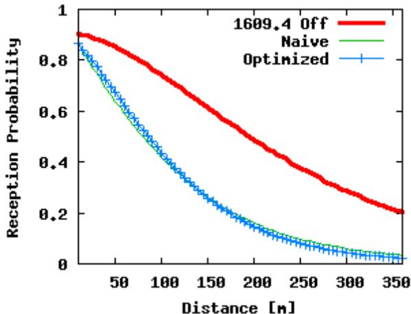
Figure 18 Safety message reception vs. distance, 150Byte, 400m, 10Hz
