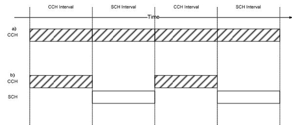
Figure 5 Channel intervals and continuous/alternating channel access
