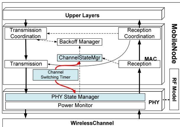
Figure 7 Modification to NS-2 simulator for IEEE 1609.4 emulation
