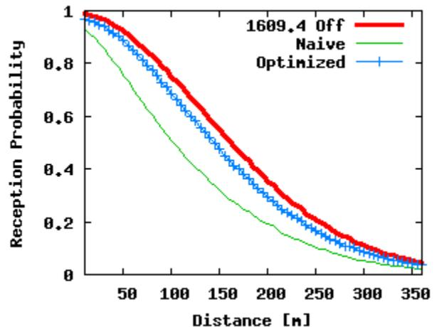
Figure 11 Safety message reception vs. distance, 75Byte, 200m, 5Hz
