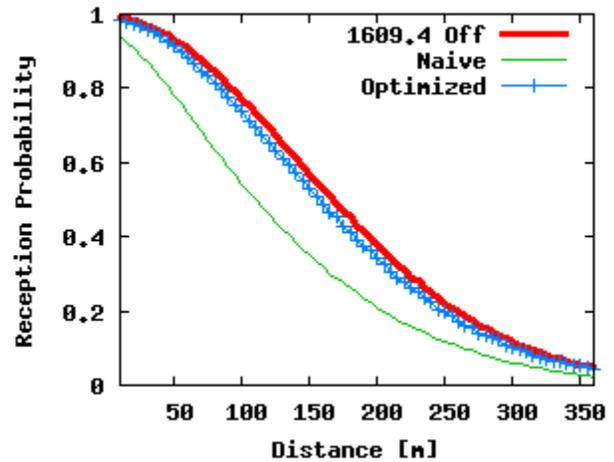
Figure 10 Safety message reception vs. distance, 75Byte, 200m, 3Hz
