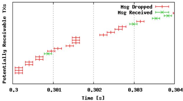
Figure 14 Synchronized collisions at the beginning of a CCH interval
