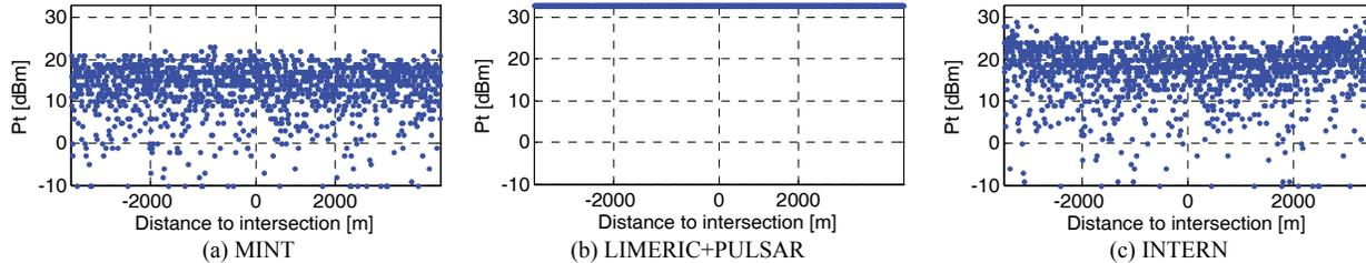
Fig. 5. Snapshot of the transmission power used by each vehicle in scenario 1 for 50 veh/km/lane after 50s of simulation time.
