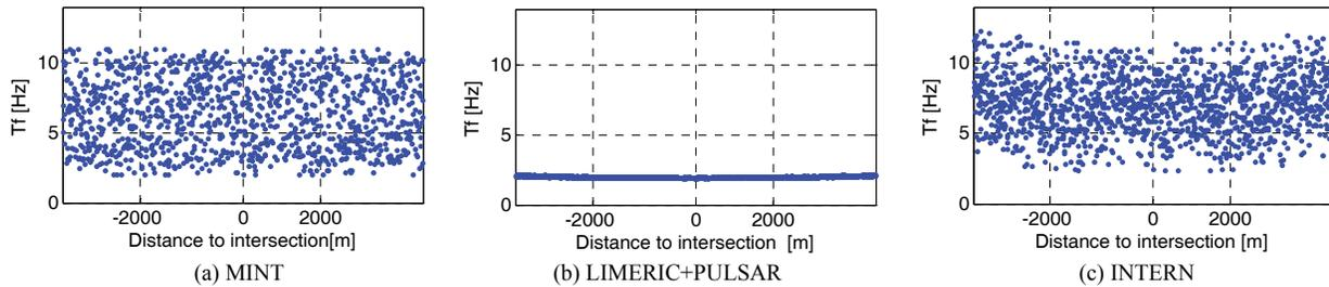
Fig. 4. Snapshot of the packet transmission frequency used by each vehicle in scenario 1 for 50 veh/km/lane after 50s of simulation time.
