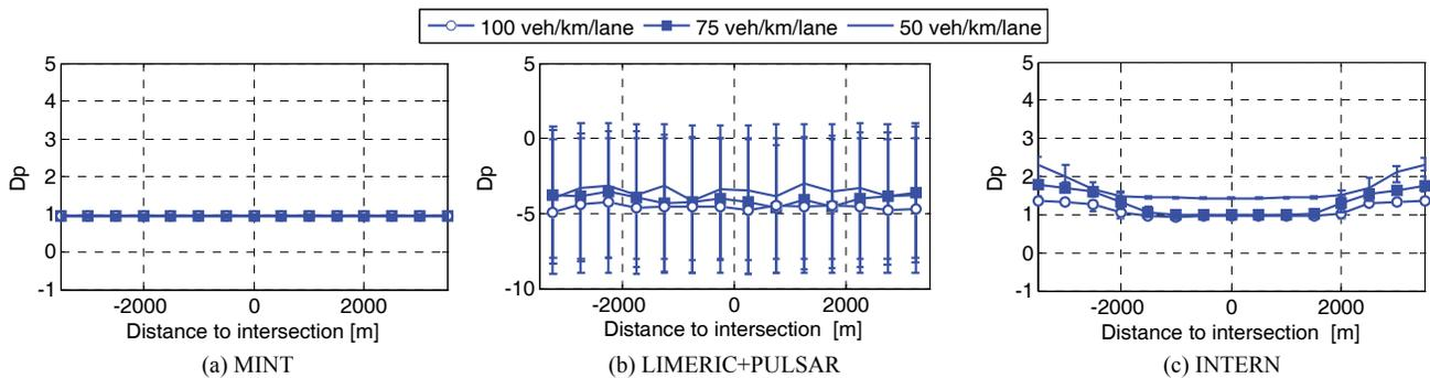
Fig. 3. Average spatial distribution of the  $D_p$  metric (difference between the number of packets per second demanded by the application and the number of packets that are received per second at the warning distance) to evaluate the application's effectiveness for different traffic densities in scenario 1. The vertical lines represent the 5<sup>th</sup> and 95<sup>th</sup> percentiles. The application's requirements are satisfied if  $D_p > 0$ .
