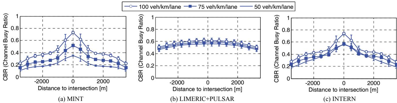
Fig. 2. Average spatial distribution of the  $CBR$  (Channel Busy Ratio) experienced to evaluate the channel load for different traffic densities in scenario 1. The vertical lines represent the 5<sup>th</sup> and 95<sup>th</sup> percentiles.
