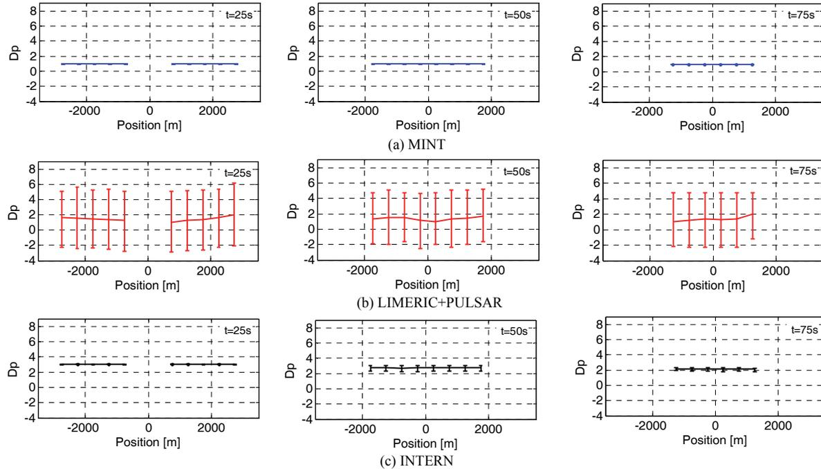
Fig. 8.  $D_p$  metric (difference between the number of packets per second demanded by the application and the number of packets that are received per second at the warning distance) to evaluate the application's effectiveness for 3 representative time instants and 50veh/km/lane in scenario 2. The vertical lines represent the 5<sup>th</sup> and 95<sup>th</sup> percentiles. The application's requirements are satisfied if  $D_p > 0$ .
