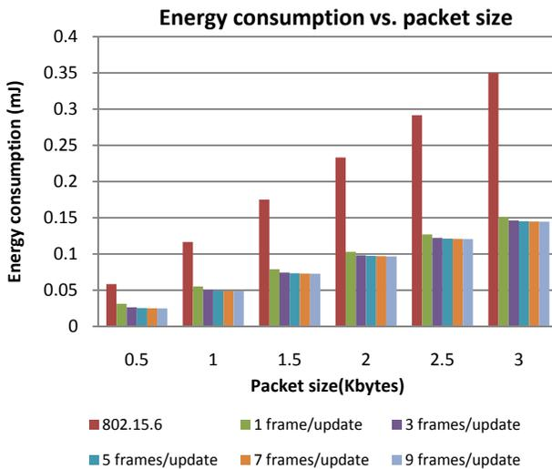
Figure 6. Energy consumption vs. packet size for proposed TDMA with different power detection interval and IEEE 802.15.6.
