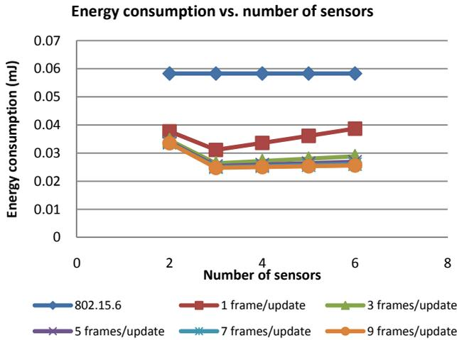
Figure 5. Energy consumption of proposed TDMA with different power detection interval and IEEE 802.15.6.
