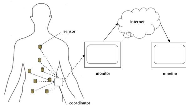
Figure 1. A simple architecture of body sensor networks.
