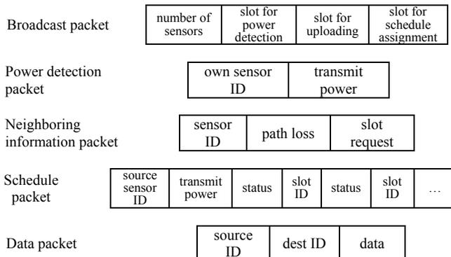
Figure 3. Data packet structure.
