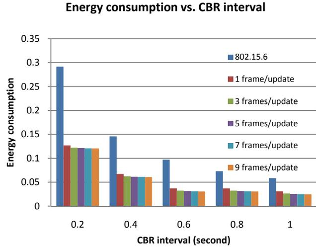
Figure 7. Energy consumption vs. CBR packet interval for proposed TDMA with different power detection interval and IEEE 802.15.6.
