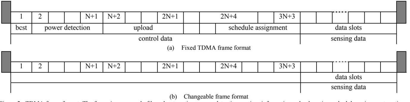
Figure 2. TDMA frame format. The frame is composed of broadcast section, power detection section, information upload section, schedule assignment section and data slots section.
