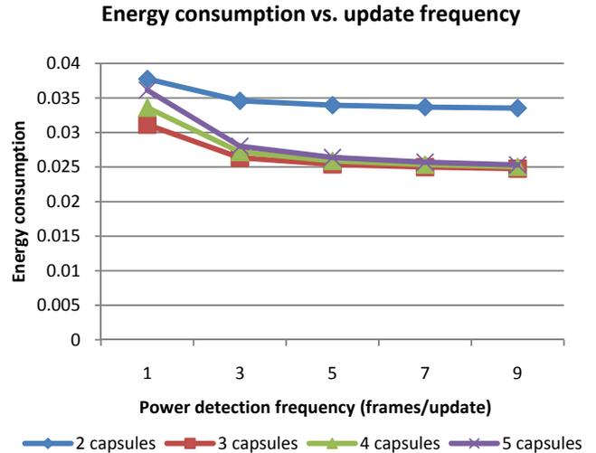
Figure 4. Energy consumption vs. power detection interval. 1frame/update represents fixed frame format. 3 – 9 frames/update represents changeable frame format.
