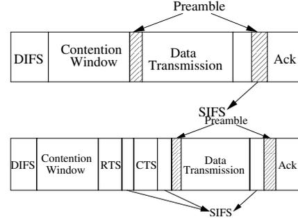
Fig. 2. Timing of an 802.11 frame transmission.
