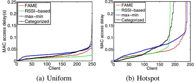
Fig. 8. Average MAC access delay of the algorithms under both uniform and hotspot distributions.
