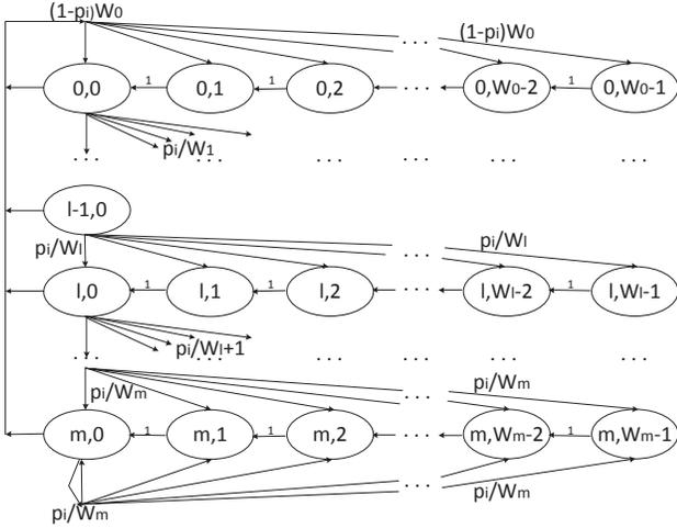
Fig. 3. Two-dimensional Markov chain model for client  $i$  with saturated traffic, where  $W_l$  is contention window size at state  $l$  and  $p_i$  is the transmission failure probability of client  $i$ .
