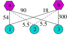
Fig. 1. An example WLAN. Nodes *a* and *b* are APs and nodes 1, 2 and 3 are clients. Lines denote the potential associations between APs and clients, and the numbers by the links are optimum data rates.
