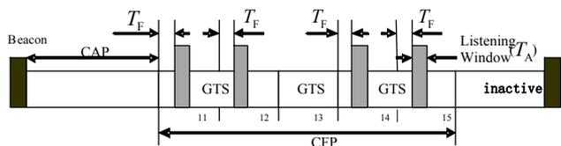
Figure 2. The Proposed Alarm Access (AAC) Superframe Structure
