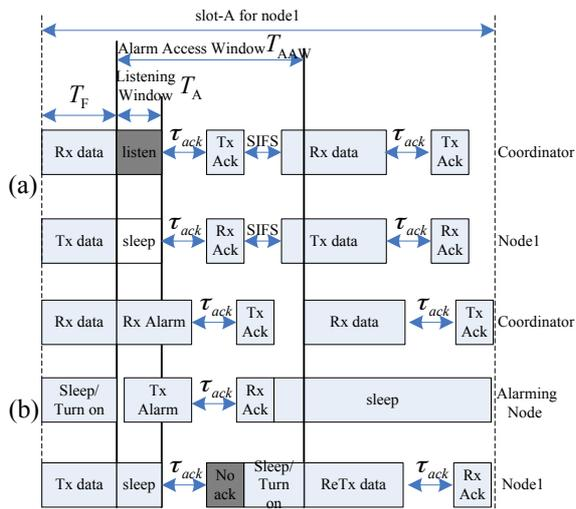
Figure 3. An Example of Emergency Data Transmission in Slot-A
