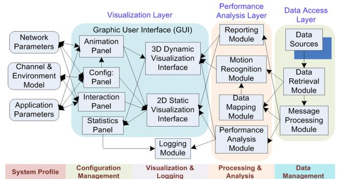
Figure 3. Software modules involved in testbed implementation
